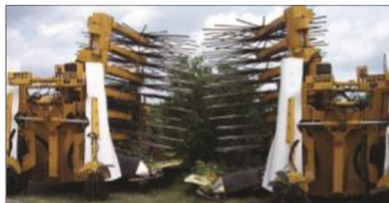
Fig 4:Continuous canopy shake and catch harvester
