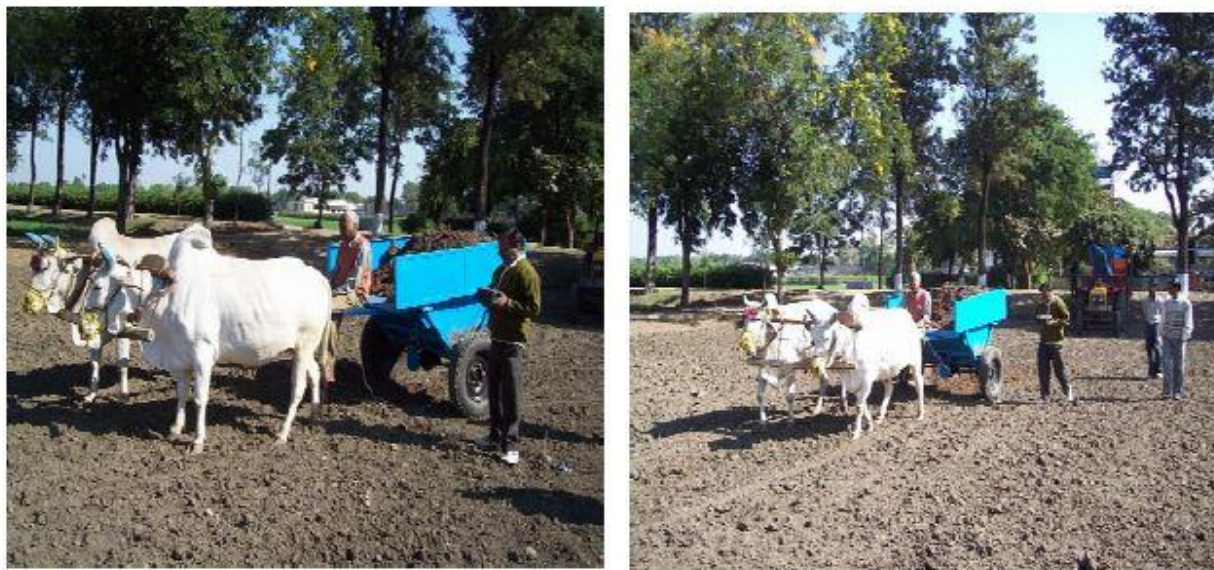
Fig.1 in field recording of pull and speed of operation with and without rotation of manure spreading auger
