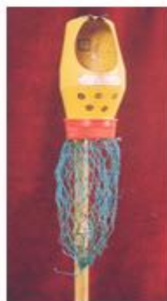
Fig 3 Manually Operated Sapota Harvester
