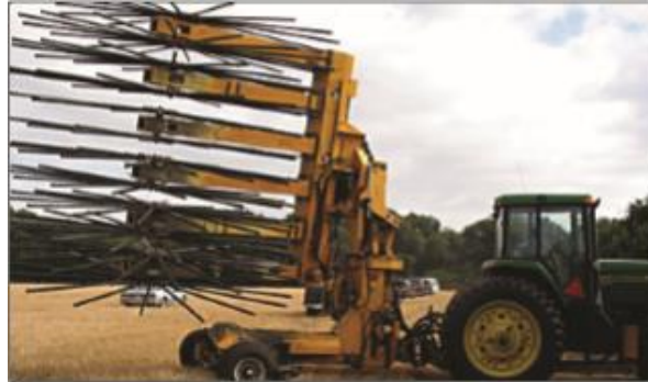
Fig 5:Tractor-drawn canopy shaker harvester
