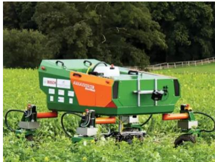
Fig.5. Bonirob farming robot (Image courtesy of Deepfield Robotics)
