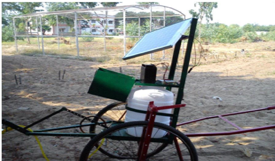
Fig 1. Trolley mounted solar operated low volume boom sprayer
