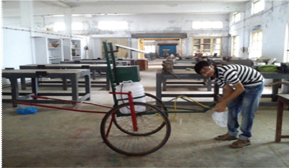
Fig 2. Calibration of solar sprayer in laboratory
