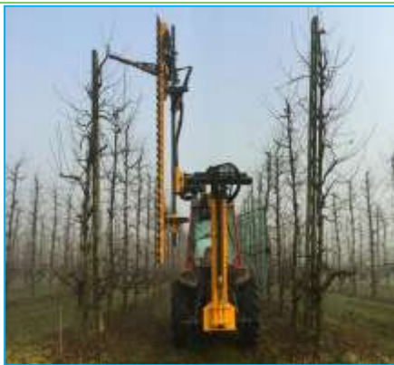
Fig: 1 Mechanical pruning system for apple trees with saw-tooth cutter driven by a tractor
