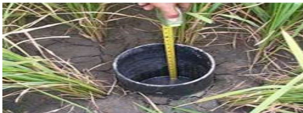
Water at 15 cm below the soil surface: Time to irrigate the field again
