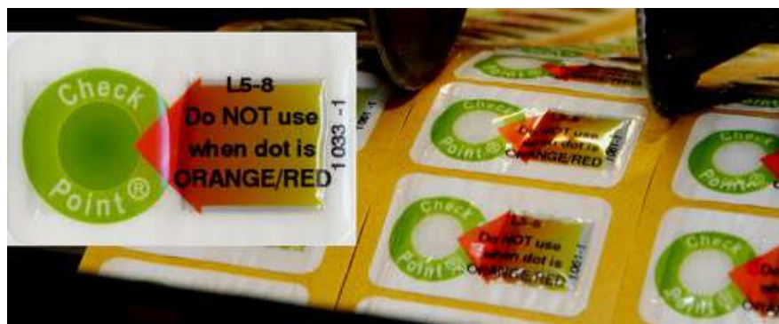
Fig 2: Time temperature indicator showing changes (Source: www.vitsab.com )
