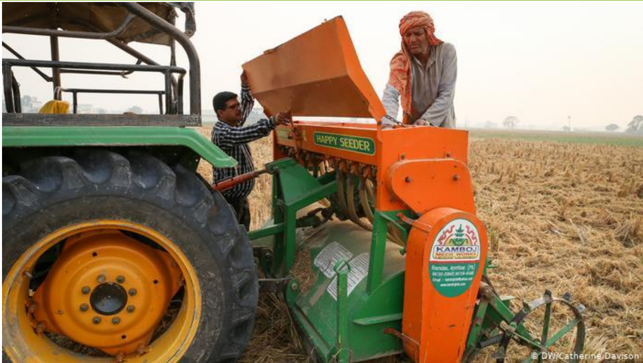
Happy seeder machine used to sow wheat in Karnal
