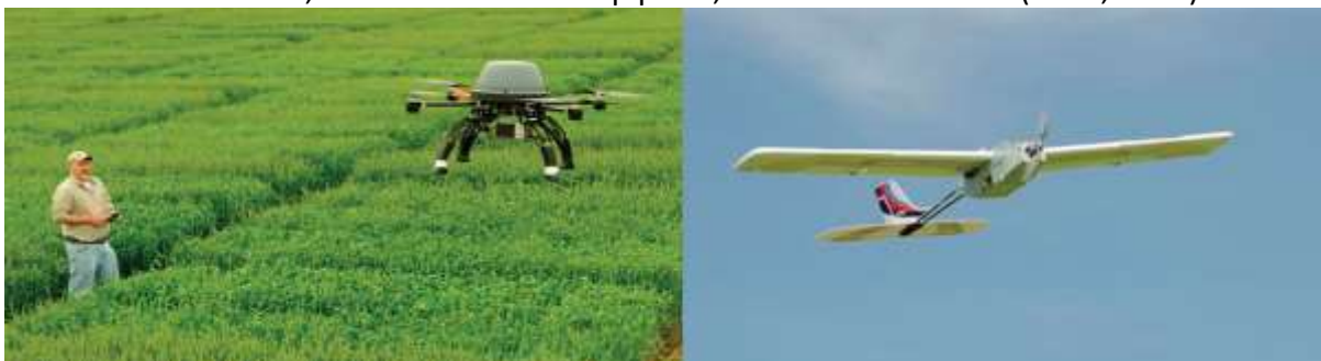
Fig1: Two types of UAVs: Rotary copter (left) and fixed-wing airplane (right)
