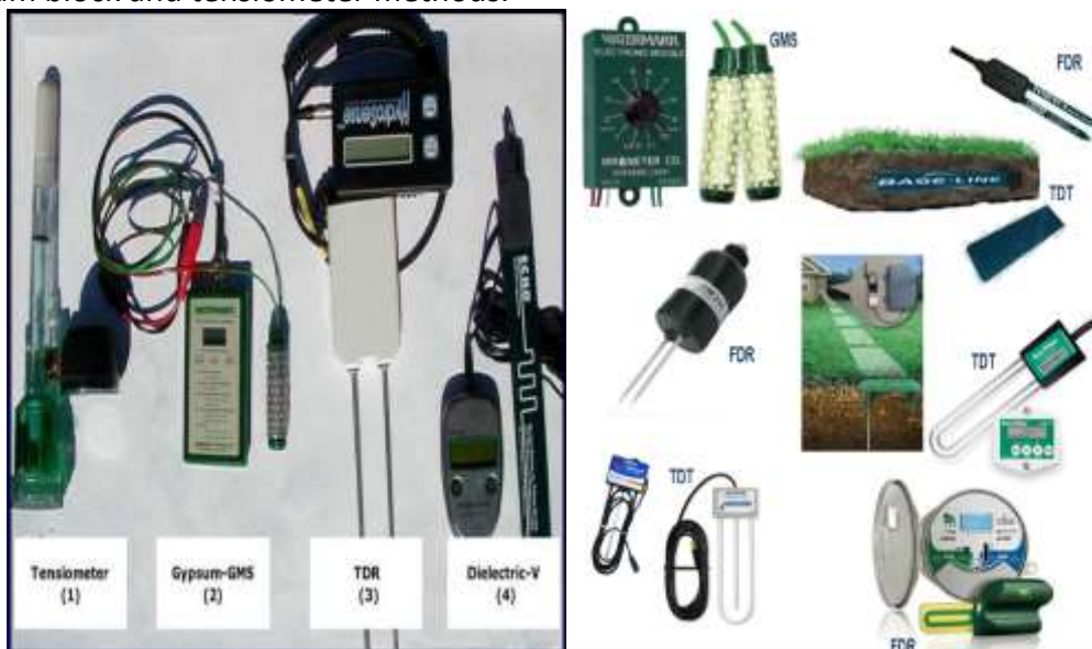
Fig 1: Different types of sensors used to estimate soil moisture
