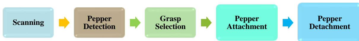
Figure 3. Functional components of harvesting robot
