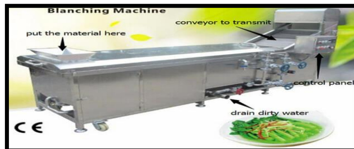
Figure 2: Hot water blancher machine.
