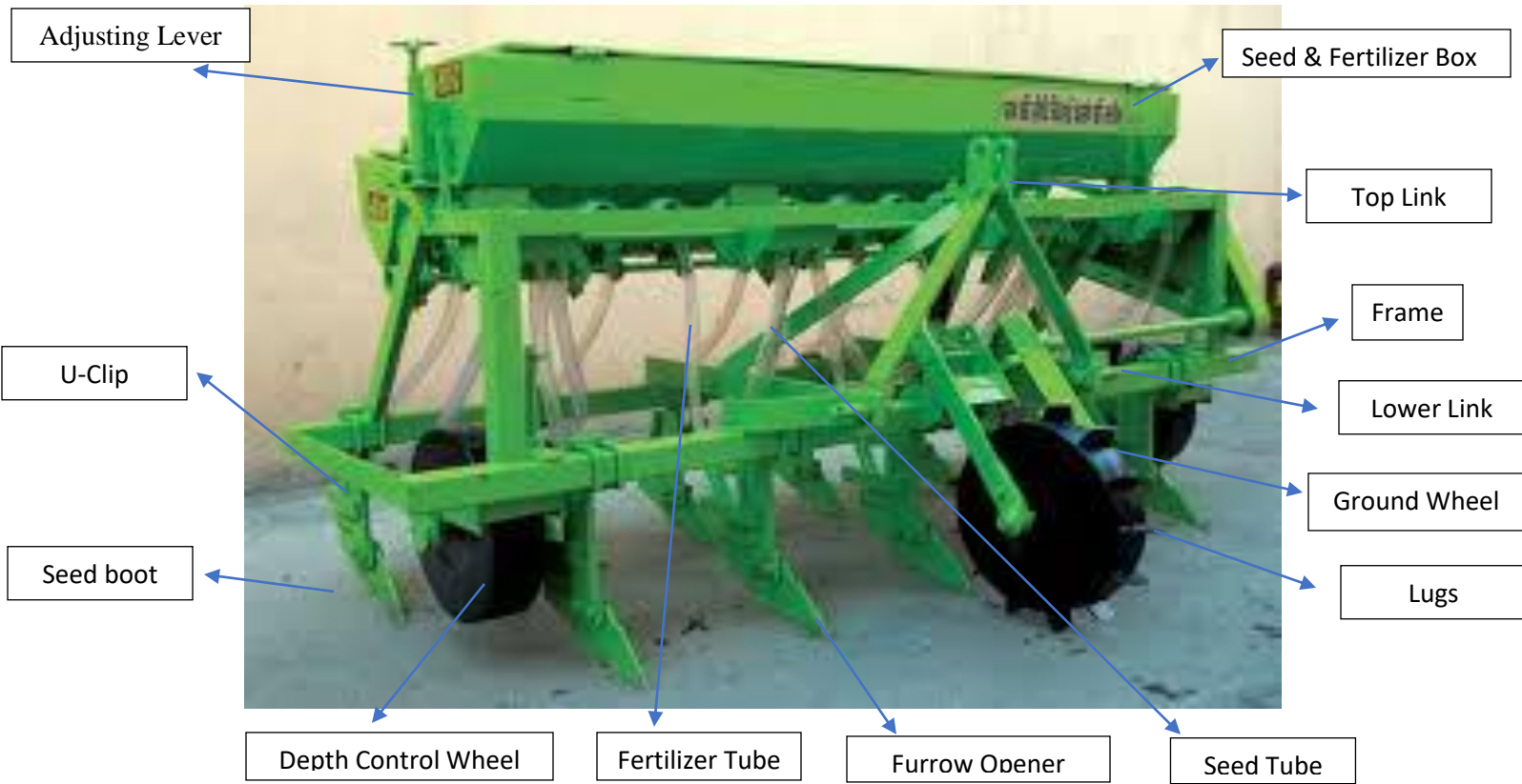
Fig. 1: Components of Tractor Drawn Multi-Crop Planter
