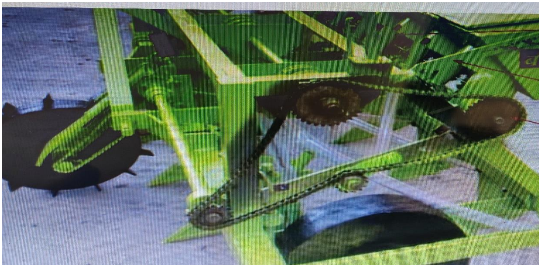
Fig. 2: Power Transmission System of Multi-Crop Planter
