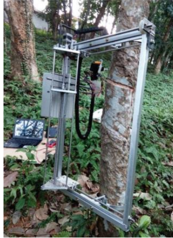
Fig. 1. Fully automated rubber tapping machine (Yatawara et al , 2019)
