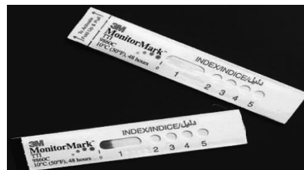
Figure 3. diffusion based 3M Monitor Mark R time temperature indicator
