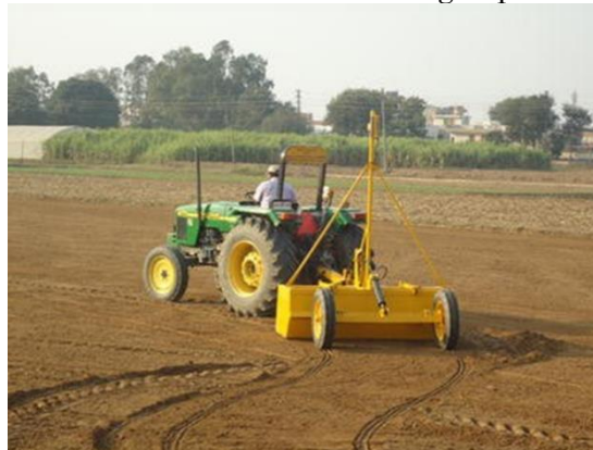
Figure.1. The view of laser land leveling (Source- https://doi.org/10.1007/s12571-015-0460-y )
