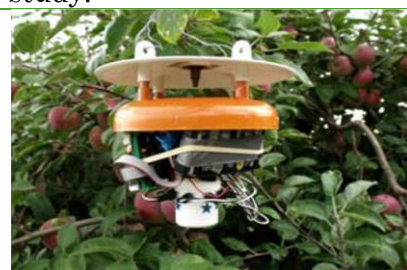
Fig 4. Electronic trap deployed in an orchard
