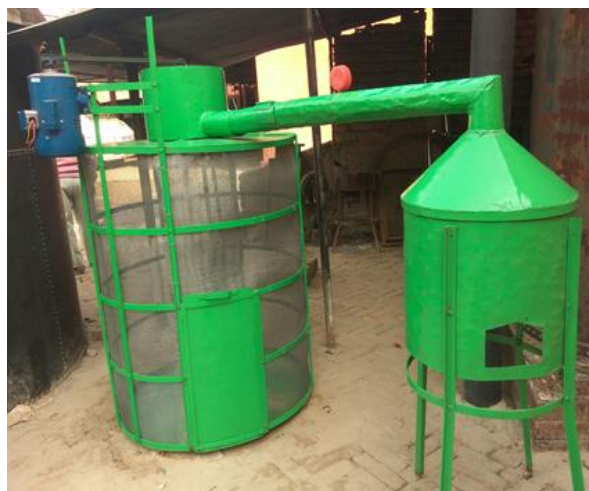
Fig. 1: Schematic and photographic view of STR dryer 1. Hollow pipe; 2. Digital temperature sensor ; 3. Pressure gauge ; 4. Digital anemometer ; 5. Gate valve ; 6. Stove ; 7. Tripod stand ; 8. Discharge gate ; 9. Outer cylindrical bin ; 10. Perforated inner cylindrical bin; 11. Motor 12. Fan and 13. Hot air.
