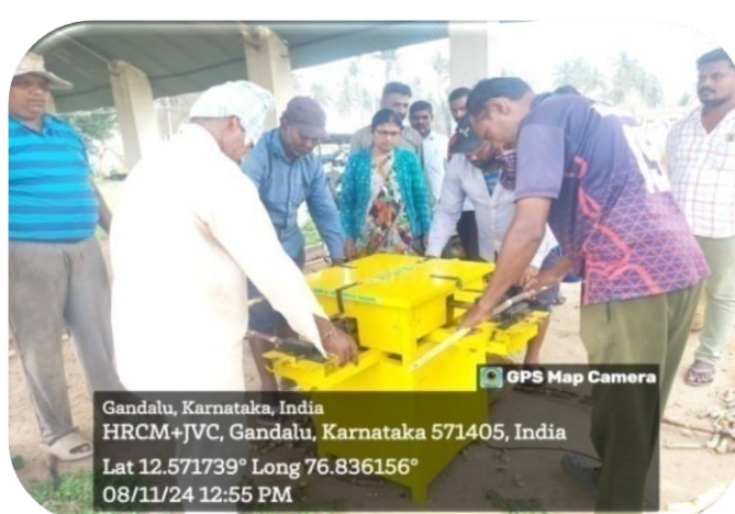
Plate 1: Cutting of single eye buds by manual method and sett cutter
