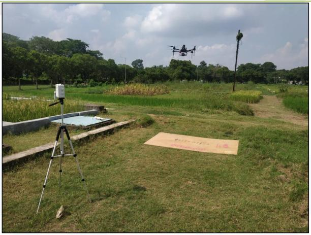
Figure 1. Unmanned Aerial Vehicle with Multispectral and Thermal Sensor
