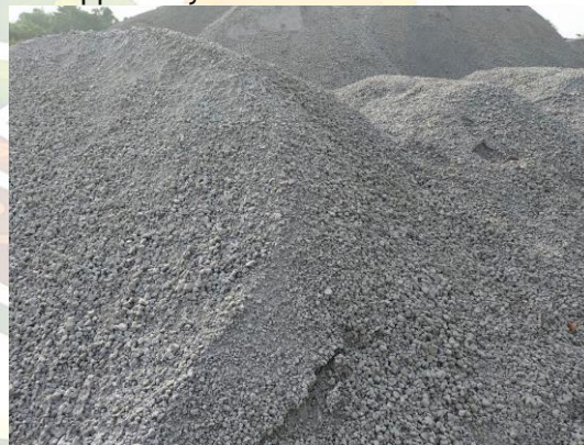
Figure 2. The powdered slag after processing
